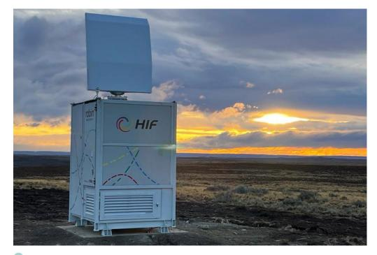
A Bird detection radar in action
