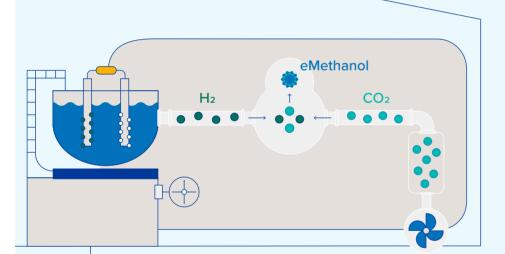
The green hydrogen is combined with the captured  $\mathrm{CO}_2$  to produce e-Methanol in a reactor through a process called synthesis. Haru Oni's methanol-synthesis unit — built by Germany's MAN Energy Solutions — uses Johnson Matthey proprietary  $\mathrm{CO}_2$ -to-methanol catalyst technology.
